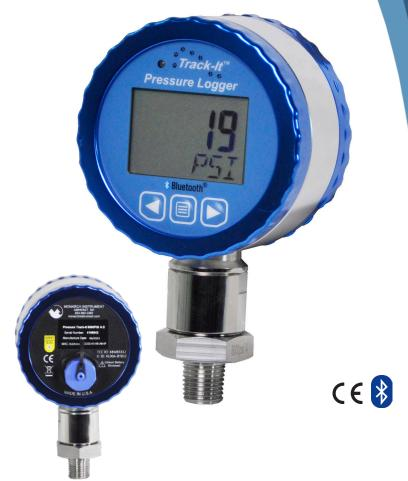
The Track-It™ Pressure/Temperature or Vacuum/Temperature Data Loggers with Display are battery-powered, stand-alone, water-resistant data loggers that emulate a pressure gauge. They can be configured to record both Pressure and Temperature up to 130,000 samples or Pressure alone, to maximize data storage space. Real-time data, alarms, and min/max information can be displayed on the multiline LCD.
